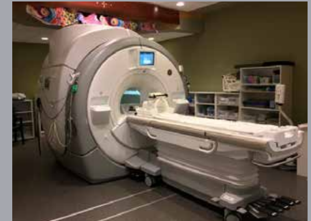
The 3T GE Discovery 750 MRI scanner located at the Lucas Center. The MRI system includes 32 channel RF coils and multinuclear spectroscopy, and provides advanced capabilities to support functional brain imaging, and imaging of the abdomen and the musculoskeletal system.
